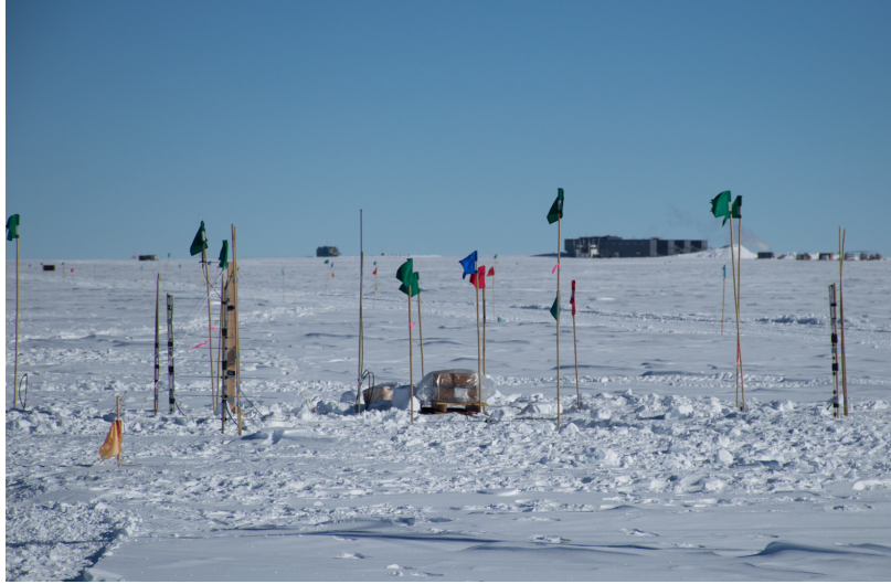
Figure 2.30: A photo ARIANNA South Pole pilot station, showing the Amundsen-Scott station in the background. Upward pointing antennas are visible, with three downward facing LPDA's and an ARA bicone antenna below the surface.
