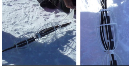
Figure 3.11: Photo of the ARA bicone antenna which is modeled in ShelfMC . Photo from [22].
